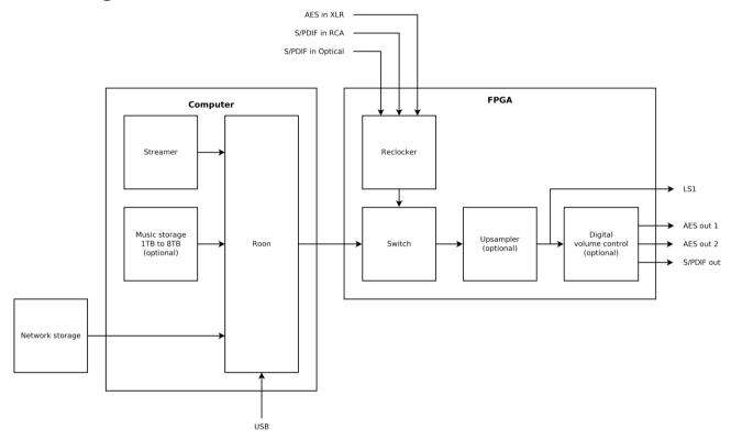
In the Block Diagram the audio flow in the MU1 is shown. As you can see, a MU1 combines the functions of a streamer, audio file server, audio file player, reclocker, upsampler and digital volume control. The audio file and streaming functions are performed by Roon Labs software. All other software is developed by Grimm Audio.
