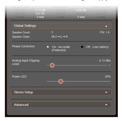
'Speaker Chain' shows how many LS1s, and in what order, are connected. The image above shows that there are two LS1s connected and the wiring goes from the MU1 to the left LS1 and then to the right LS1. In a surround setup with LS1s the indicated chain is important to double check, see chapter Stereo system wiring for the proper surround setup wiring. In this chain 'LS' means Left Surround and is the Rear Left channel, 'RS' is the Rear Right channel, 'C' is the Center channel.
